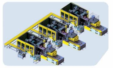
Flexible Automation -360° visual detection, robot operation, automatic 02 assembling, parts insert, polishing and deburring... Visual Detective System
