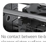
No contact between tie-bar and moving platen, cleaner platen surface and less pollution
