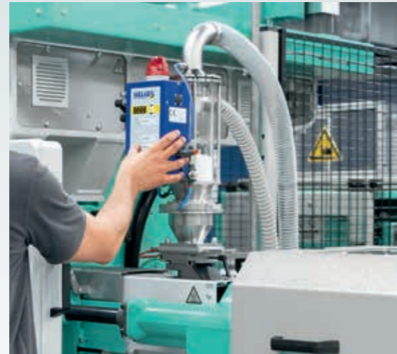
Due to their compact construction, HELIO® Clean dedusting units can be mounted directly on the injection moulding machine or a drying container.
