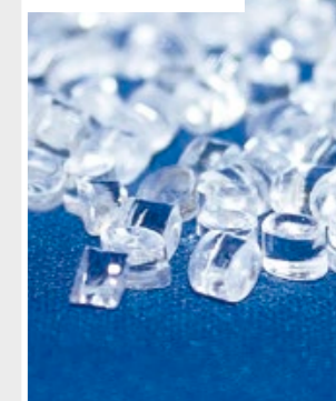
PMMA raw granulate before and after dedusting.
