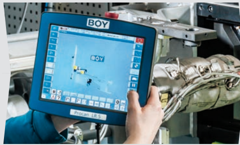
Mobile 10" terminal with cabled emergency operation and enabling switches
