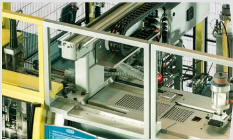
Assembly of the BOY-Handling LR5 onto the injection moulding machine
