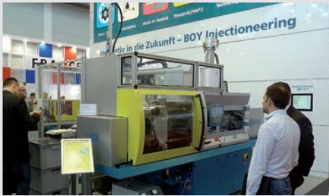
Production cell with individual safety housing
