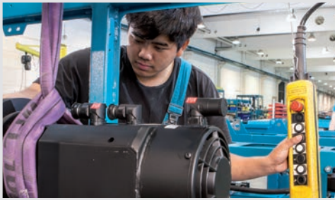
“Heart” of the insert moulding machine: The efficient servo-motor pump drive
