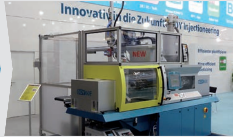
Production cell with CE-compliant safety housing
