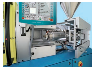
The swivel-out injection unit facilitates alterations and maintenance
