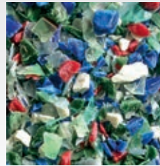
grinding material from shredder
